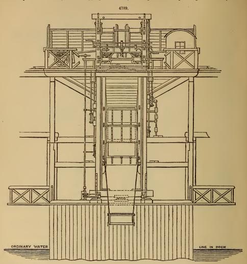
as possible, merely letting the coals slide sufficiently down to allow of the next wagon being teamed; so that though in the first filling of the spout, or on altering the level of the spout, the coals have a few feet to fall, yet this only applies to a small quantity of coal. Afterwards the whole mass descends slowly, and no further breakage takes place. When these points are carefully attended to, as little breakage takes place by this system as by any other.
